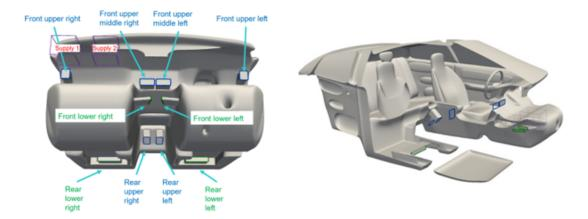
Figure 52: Inlets to the cabin geometry and air supply locations from the blower.
