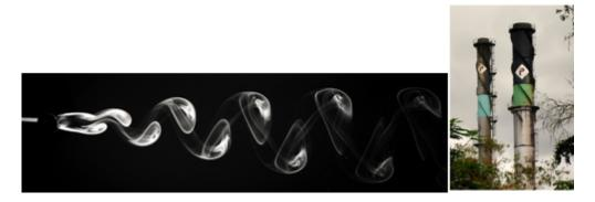
Figure 19: Vortex Shedding Formation Downstream of a Cylinder (left) and Chimney with Spirals (right)
