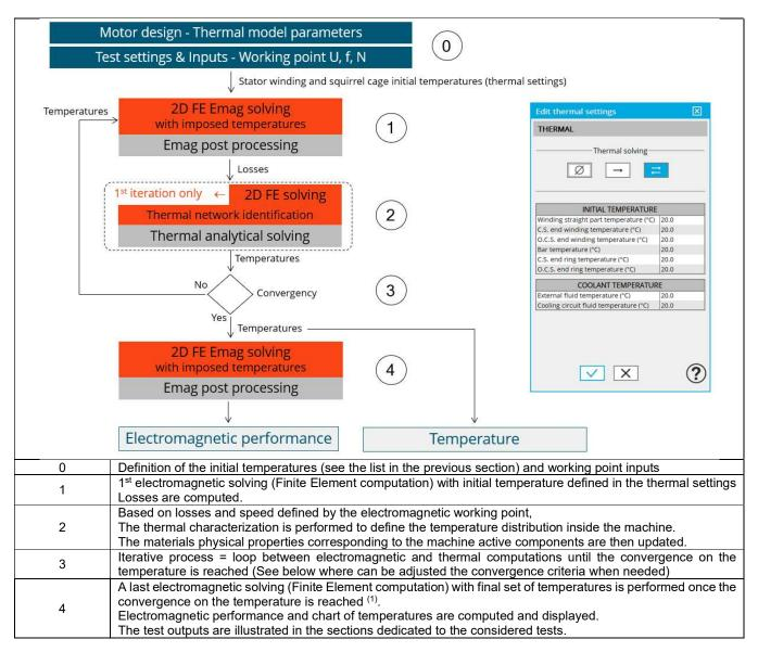
2) The temperatures which are considered for computed the final machine performance (step 4 in the previous flow chart) can be read in the table dealing with "Winding and Squirrel cage characteristics" of the test configuration at the beginning of result report. See below illustration. The same principle is applied for the squirrel cage temperature.
