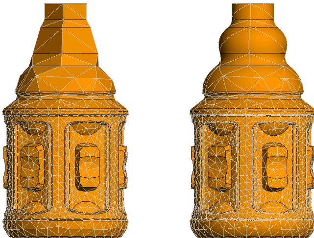
Figure 320: A model with flat triangular mesh (on the left) and with curvilinear mesh and higher order basis functions enabled (to the right).
