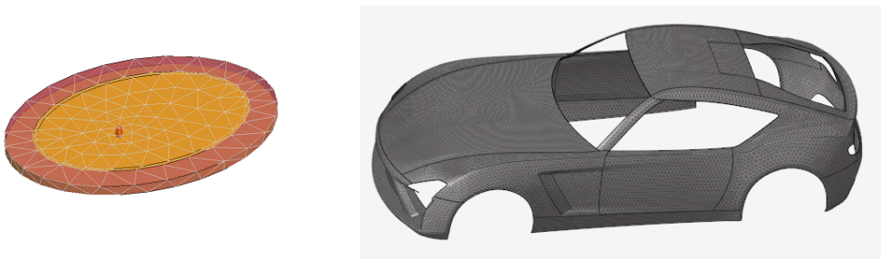
Figure 993: On the left, the circular patch antenna. To the right, the platform (vehicle) model meshed with HyperMesh. Images not to scale.
