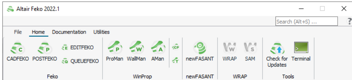
Figure 570: The Launcher utility allows quick access to Feko, WinProp (Microsoft Windows only), newFASANT, WRAP components (Microsoft Windows only), documentation and utilities.
