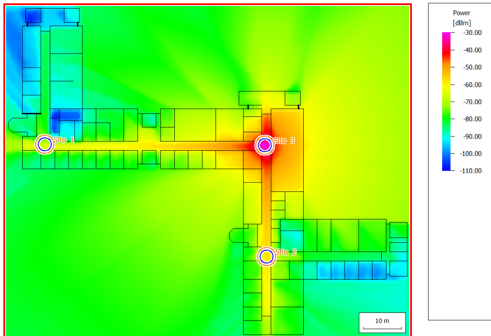
Figure 180: Power calculated for Site 3 Ant 1 using the DPM.
