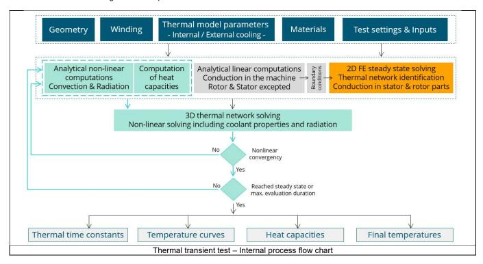
The inputs of the internal process are the parameters of:
