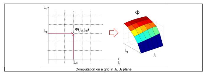
Our modeling considers cross-saturation. However, neither winding harmonics nor the variation of reluctance as a function of angular position of the rotor are considered.
