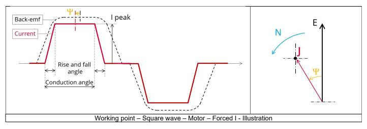
All the results are computed from a Finite Element Analysis (Flux) - Transient application. The results of this test give an overview of the electromagnetic behavior of the considered motor.
