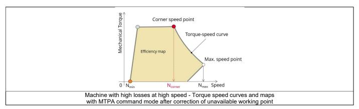
So, when the targeted working point is in an unreachable zone (left or right white area of the figure above), a warning message is issued by FluxMotor® and the efficiency is set at " - ". All other computed results are available and can be analyzed (power balance) for targeting a reachable working point.
