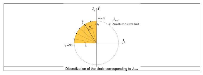
Then an optimization process is performed to get the base speed point which corresponds to the working point at maximum line current and maximum line-line voltage:  $I = I_{max.}$  and  $U = U_{max.}$
