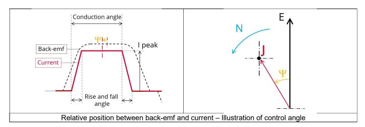
The two previous figures show the parameters defining the line current (I peak, control angle, speed, conduction angle, rise and fall angle). The resulting line current is then applied in a transient simulation (with the Finite Element Analysis software – Flux®): the phase current, the phase voltage, Line-Line voltage, the electromagnetic torque, useful torque, and the losses are outputs of this transient simulation.
