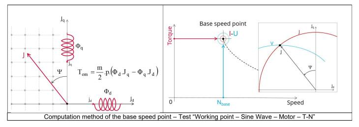
Note: We remind that for the base speed point, both commands "MTPA and MTPV" lead to the same results. In fact, the base speed point corresponds to the working point which maximizes the mechanical torque at maximum current and at maximum voltage. Following this, we easily understand that we will obtain same results with MTPV or with MTPA.
