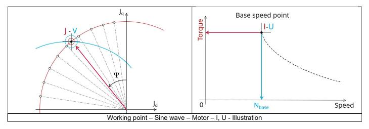
The results of this test give an overview of the electromagnetic analysis of the motor considering the machine topology. The general data of the machine, like machine constants, power balance and magnet behavior are computed and displayed. The magnetic flux density is also computed in every region of the machine's magnetic circuit to evaluate the design. In addition, ripple torque at the base speed point is computed.
