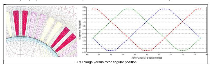
The time variation of the phase voltage is deduced by derivation of the flux linkage. It is performed by considering the following formula:
