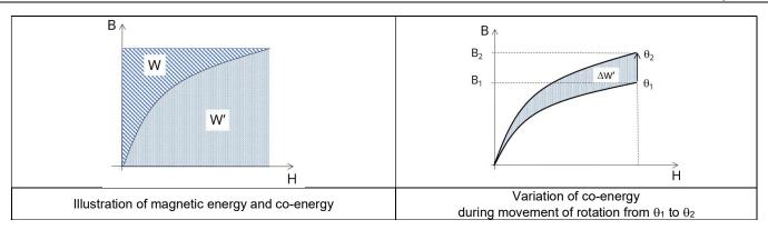
Depending on the position of the rotor (from  $\theta_1$  to  $\theta_2$ ), the reluctance of the system changes, causing a variation of magnetic flux density, represented by the colored area  $\Delta W'$  on the right graph. This area represents the variation of the co-energy when moving from  $\theta_1$  to  $\theta_2$ .
