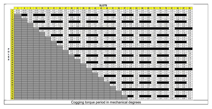
Note: An extremely small cogging torque period implies the need of a very thin mesh to get accurate results (by using a low airgap mesh coefficient value – See advanced parameter definition). Thus, the number of elements in the corresponding model will be very high (it means a high mesh density).
