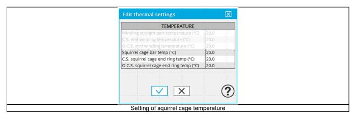
It is possible to define temperature of the three main parts of the squirrel cage:
