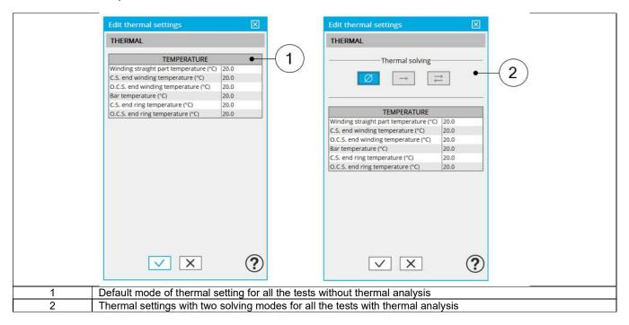
In the current version, the tests which allow using the thermal solving mode are the computations of working points defined by U, f, N with motor convention for Induction Machines with Squirrel cage with inner rotor only.
