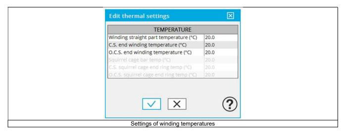
It is possible to define temperature of the three main parts of the stator winding:
