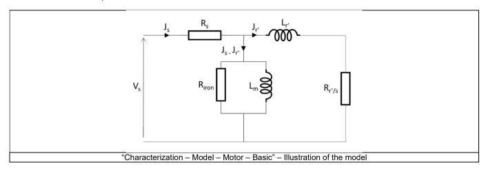
Warnings! The resulting model is a linear one, so it cannot provide accurate results on the whole ranges of operating voltages and frequencies.
