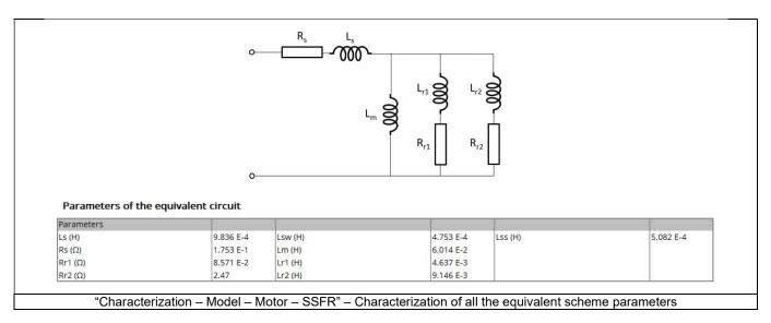
These results are based on the magnitude and the phase of the operational inductance transfer function which are computed with Finite Element software Flux® 2D.
