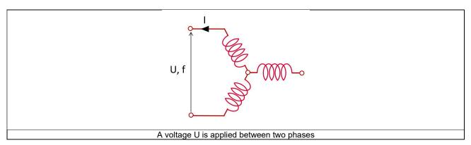
The operational inductance transfer function is deduced from the applied voltage and frequency as follow:
