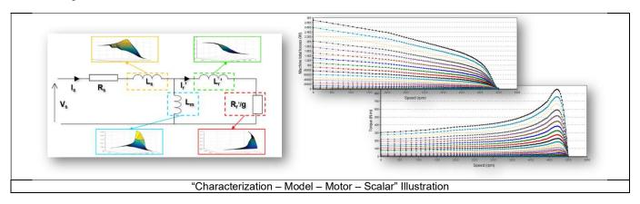
The results of this test give an overview of the electromagnetic behavior of the machine considering its topology. For a set of Line-Line voltages (U) and a set of power supply frequencies (f), the general parameters of the machine like, mechanical torque, currents, power factor and power balance are computed and displayed as curves.
