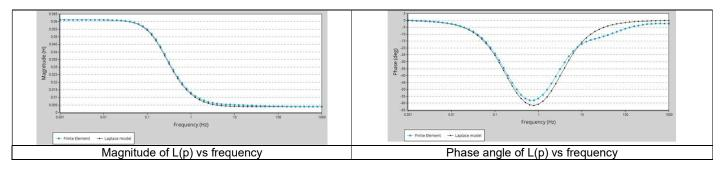
In this case, the first order is not enough accurate to make the resulting model correspond to the considered motor frequency-response.
