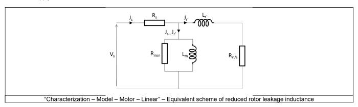
$V_s$ : Stator phase voltage at the frequency " $f_s$ ". Stator phase current at the frequency " $f_s$ "
