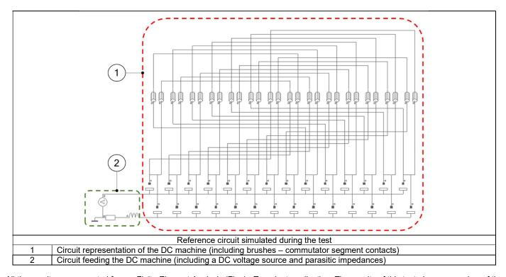
All the results are computed from a Finite Element Analysis (Flux) - Transient application. The results of this test give an overview of the electromagnetic behavior of the considered machine at a given working point.
