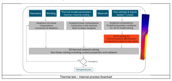
The inputs of the internal process are the parameters of: Geometry, Winding, Internal cooling, External cooling, Materials, Test settings and inputs.
