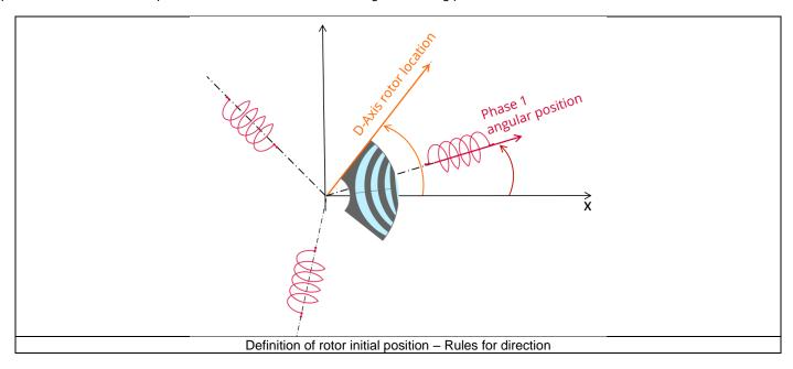
The winding axis of the reference phase is defined from the phase shift of the first electrical harmonic of the magneto motive force (M.M.F.).
