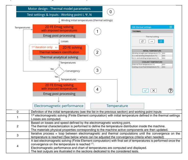
(1) The temperatures which are considered for computing the final machine performance (step 4 in the previous flow chart) can be read in the table dealing with "Winding characteristics" of the test configuration at the beginning of result report. See below illustration.
