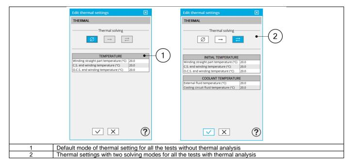
In the current version, the tests which allow using the thermal solving mode are the computations of working points defined by I,  $\Psi$ , N with motor or generator convention for Reluctance Synchronous Machines with inner rotor only.
