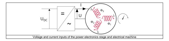
The chosen inverter control drives the ratio between the DC bus voltage and the line-line voltage seen at the machine terminal. This ratio is defined as:
