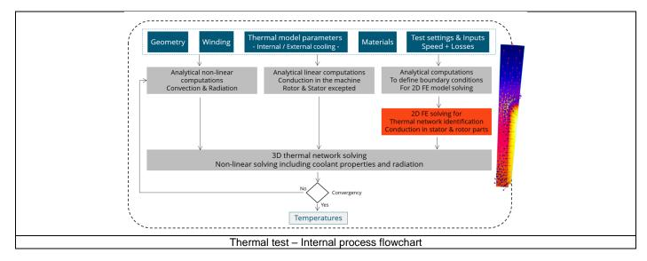
The inputs of the internal process are the parameters of: Geometry, Winding, Internal cooling, External cooling, Materials, Test settings and inputs.
