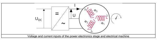
The chosen inverter control drives the ratio between the DC bus voltage and the line-line voltage seen at the machine terminal. This ratio is defined as:
