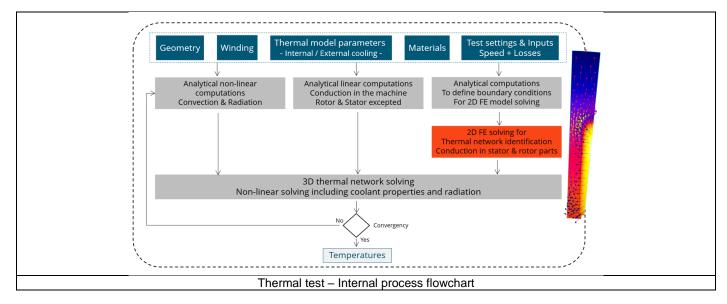
The inputs of the internal process are the parameters of: Geometry, Winding, Internal cooling, External cooling, Materials, Test settings and inputs.
